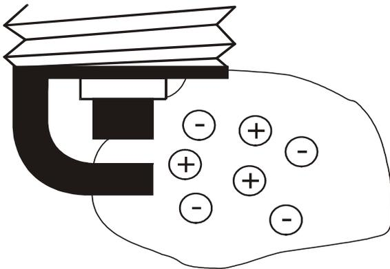
After end of sparking, a test voltage of 1 kV (resulting from 23 V auxiliary voltage) is applied to the spark plugs between the center and ground electrodes.
