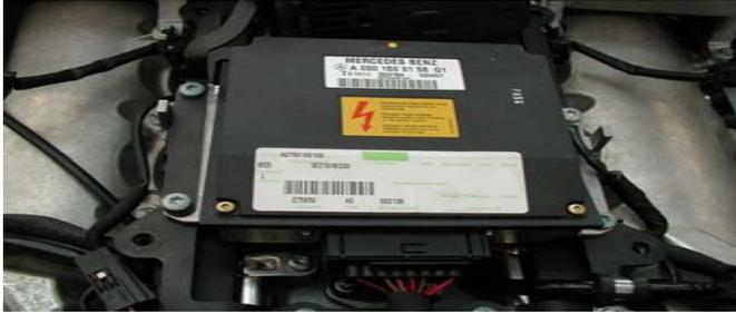
The power supply unit operates as a DC voltage supplier, the function of which could be compared to that of a power station.
