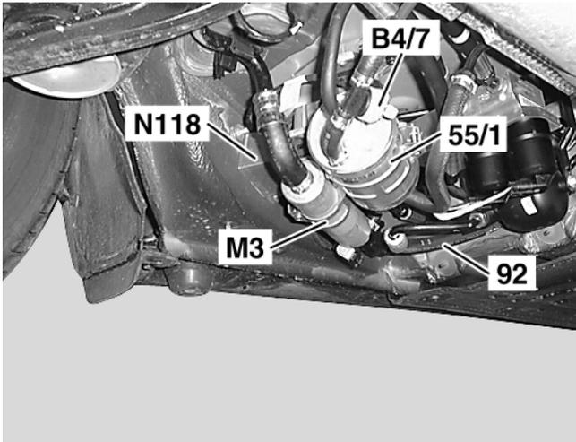
In order to prevent any increase in temperature in the fuel tank caused by the heated-up fuel return flow, vehicles with the 275 and M285 engines also have the fuel system designed as an induction system.
