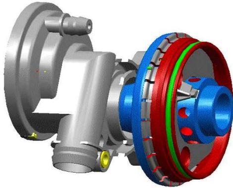
At a specific vacuum ( $> 50$  mbar) in the charge air manifold the connection to the crankcase is sealed by means of a diaphragm in the pressure regulator valve.
